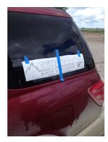
Step 2: Position your graphics and tape into place using a strip of tape to act as a centre hinge.
