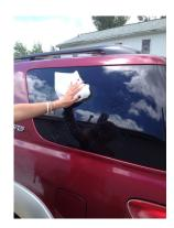
Step 1: Prep the surface using soapy water to remove any dirt and grime that may be on the surface. You can use isopropyl alcohol to remove any sticky residue. Make sure surface is dry.
