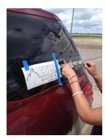
Step 4: Starting from the centre, slowly apply the graphics to the surface using a squeegee or credit card. Be sure to work your way from the centre out in small strokes taking "little bites".
