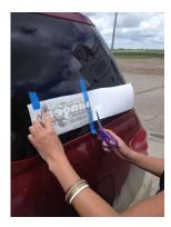
Step 3: Peel the graphics back to your centre hinge and cut the wax backing off.
